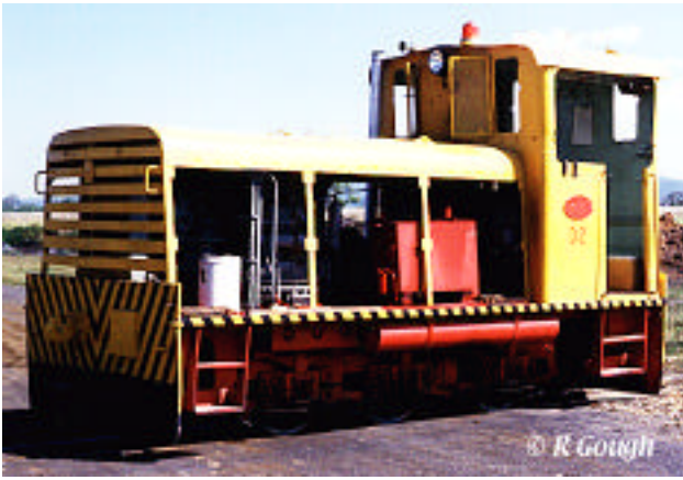
Bundaberg Jenbach D2 at Eton Sugar Mill c.1970 fitted with Gardner motor; as seen in Gough and Webber (p 18 top).
